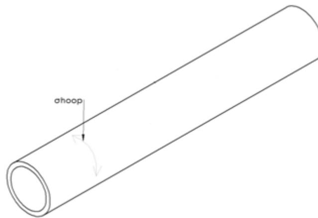
Figure 1 – Stress from internal pressure
