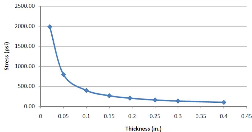
Figure 2: Hoop stress as a function of tube wall thickness
